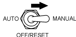
Figure 39. Auto-Off/Reset Manual Switch (Manual Position)
