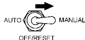
Figure 38. MPEC Control Switch (Manual Position)
