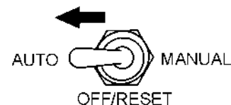
Figure 52. MPEC Control Switch (AUTO)
