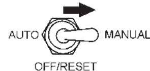
Figure 38. MPEC Control Switch (Manual Position)
