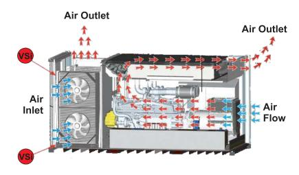
The FQ series generators by TecnoGen incorporate their Patented VSi technology. VSi (Variable Speed invertor) technology uses variable speed electric fans to manage the cooling for the generator instead of standard engine driven fans, which steal power from the engine and create excessive noise.
